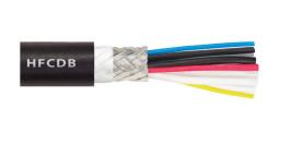
9.2mm Low-Profile Diameter High Tensile Strength Tight Buffer SMPTE 311M-2009 Compliant Directional Arrow Printed on Jacket Easy-to-Pull Through Conduit Direct Burial Construction
